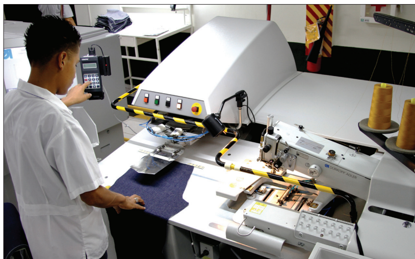
At General Sportswear's Sincotex factory in Nicaragua, an operator uses a CGS BlueCherry terminal and a sewing machine with an automated back pocket setter.
